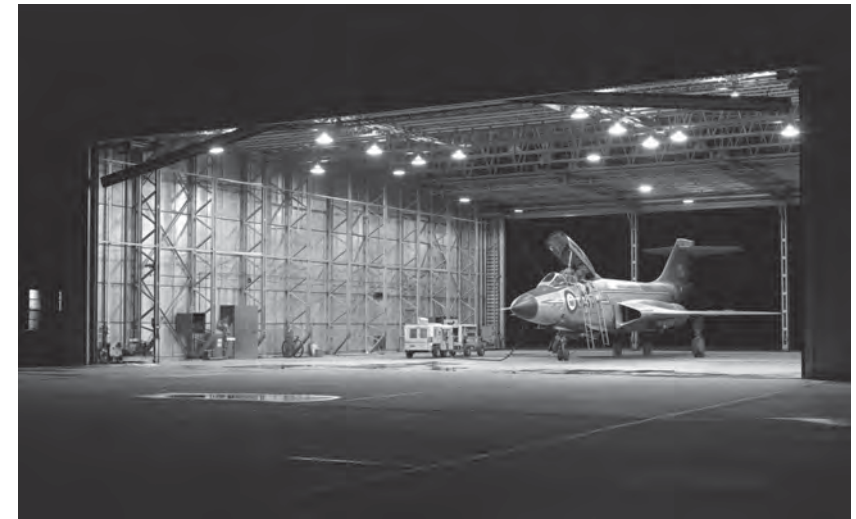
This is a CF-101B in a Quick Reaction Alert facility equipped with Falcon air-to-air missiles sometime in the early 1960s before MB-1 Genies were stored in Canada. [Department of National Defence]
