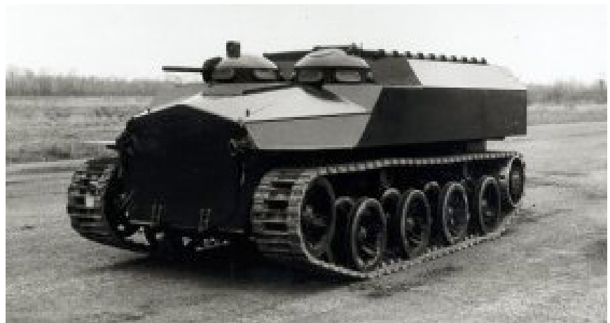
Canada’s first multi-role combat vehicle, the “Chassis Tracked, Light” (better known as the Bobcat) in its basic form featuring a cupola-mounted machine gun and a roll-back armoured roof, from which the eleven infantrymen mounted in the back compartment could fight. (Courtesy CFPU)
