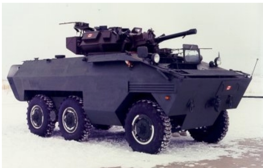
Brazil's Urutu armoured car, when equipped with a modified Alvis Scorpion turret and 76 mm gun, became another serious contender for the AVGP in 1976. (Courtesy CFPU)
