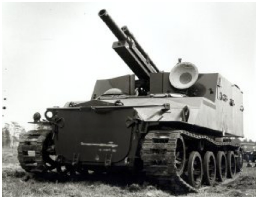
The 105 mm self-propelled gun version of the Bobcat. This vehicle, like the rest of the family, was designed to be air-portable using the RCAF's C-119 transport aircraft. (Courtesy CFPU)
