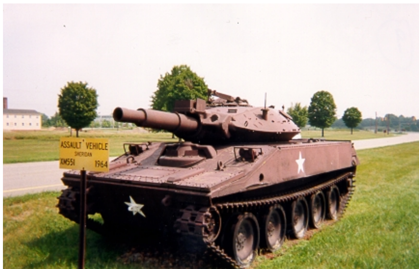
The move towards air-portability in the 1960s focused attention on air-portable armour. The main vehicle of interest was the American Sheridan, equipped with a 152 mm gun/missile launcher, which could be carried in C-130 aircraft. The vehicle proved to have serious deficiencies in the low intensity environment of Vietnam. (Author’s Collection)
